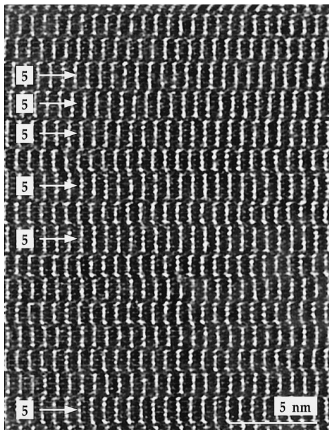
FIG. 16. HREM image in the [1\ 1\ 0] orientation showing the combination of stacking disorder and disordered chemical intergrowth. In both the orthorhombic (lower part) and the monoclinic (upper part) domains, layers consisting of 5-membered clusters (marked by arrows) are randomly intergrown.
